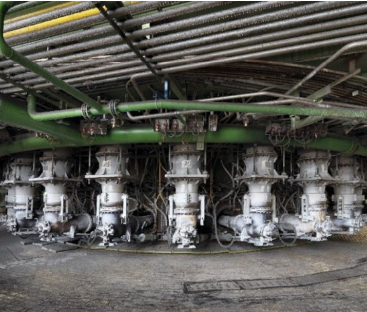
Tuyeres for hot air injection at the blast furnace
